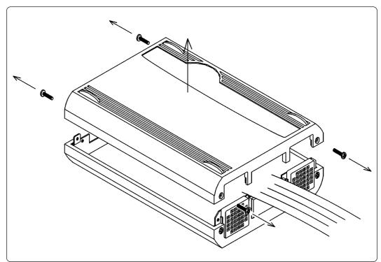
Figure 3.1 Removing the upper cover
